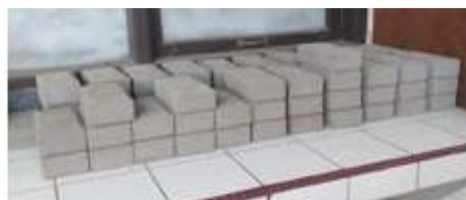
Gambar 5. Perawatan Paving Block
