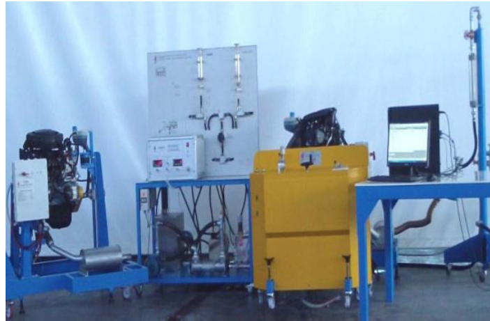
Gambar 2. 3D T101D automotive engines test bed, with optional
