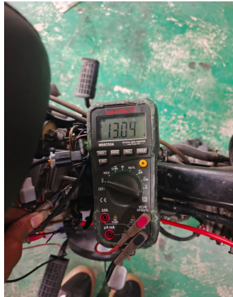
Gambar 2. Pengecekan Tegangan Regulator Fullwave
