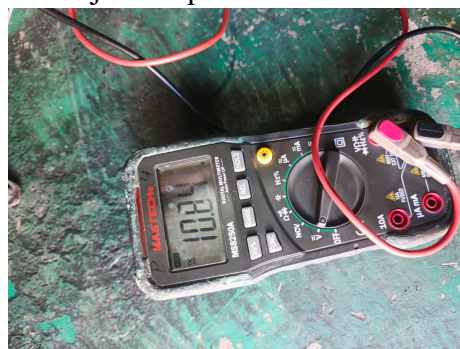
Gambar 1. Pengecekan Tegangan Regulator Halfwave
